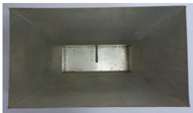
Fig.10. Photograph of fabricated pyramidal horn antenna.
